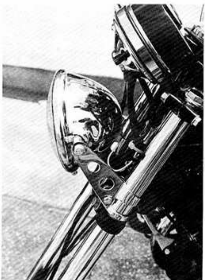
Variation on ear type is this clamp-on ear mount that is adjustable for height.
