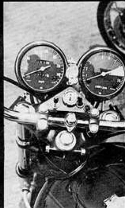
Moving switches up on handlebar eliminates some clutter.
