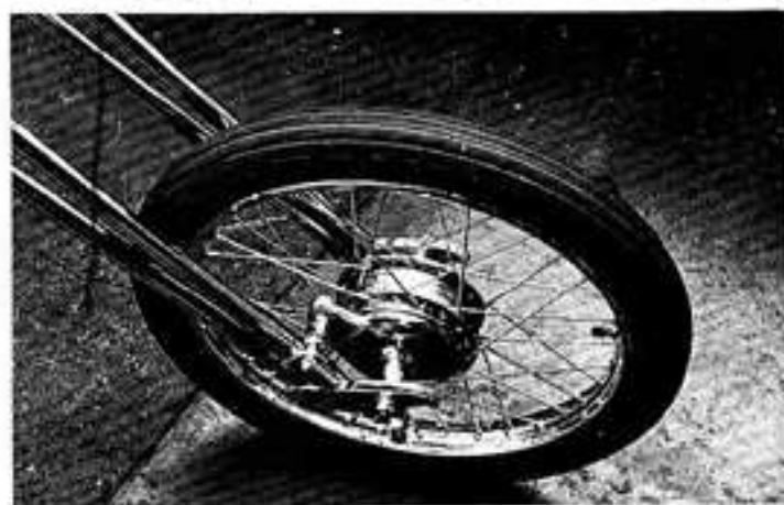
Standard drum looks good if heavily chromed up. Extra braking from big drum is a good safety factor.
