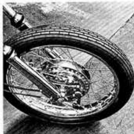
On girder forks, anchor the drum brake directly to the leg. (This happens to look like a springer.)
