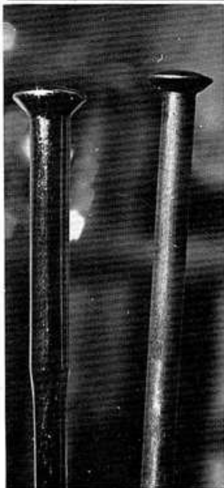
Some hubs require a straight spoke. This is strongest type.
