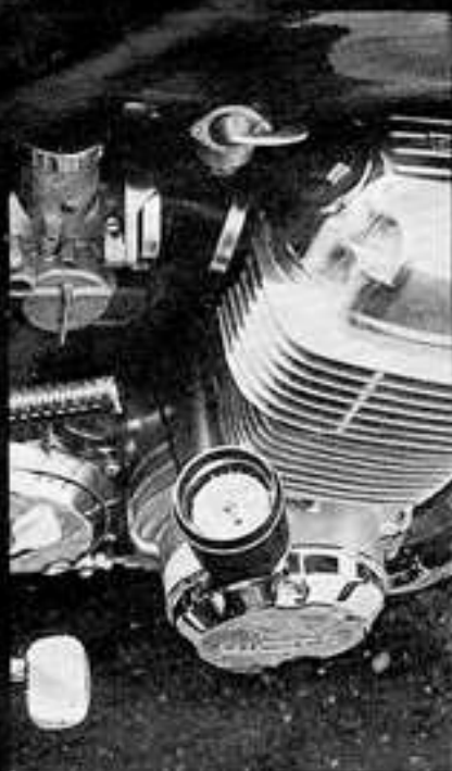
Illuminated oil pressure gauge keeps an eye on the engine's internals.
