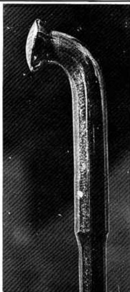
Tapered spoke has 9 ga. head and tapers down to 10 ga.
