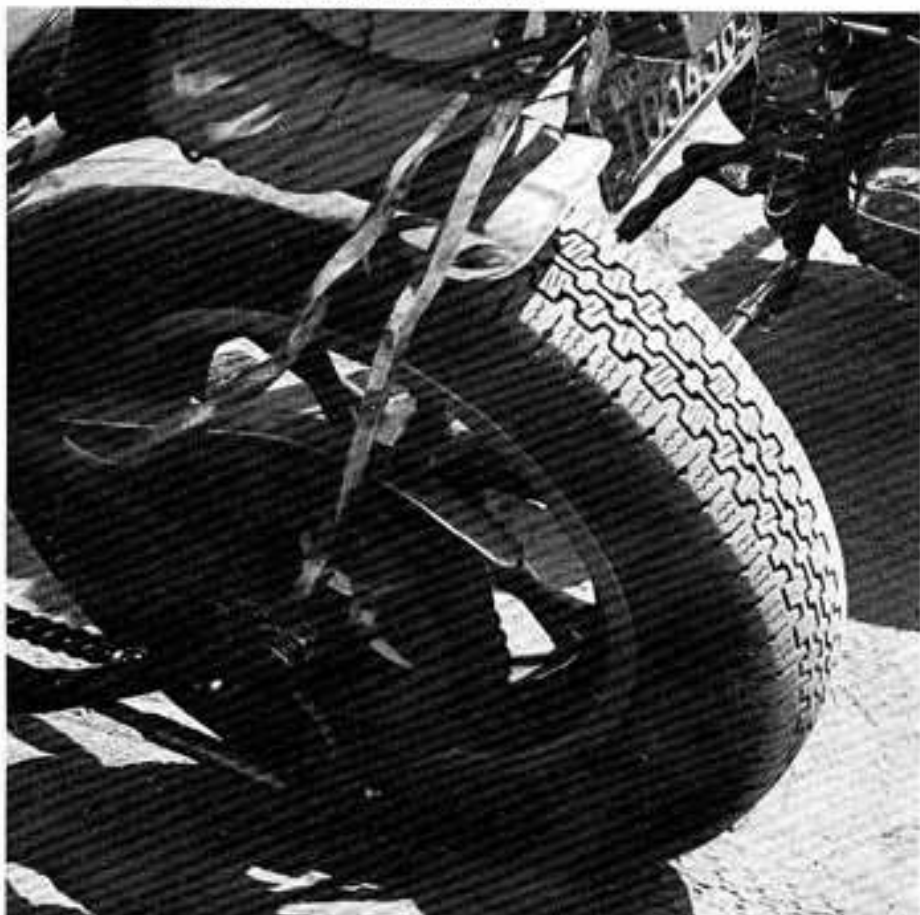
It's not a good idea to use an automotive tire on a bike. This Pirelli tire has a slightly rounded tread — works fair.
