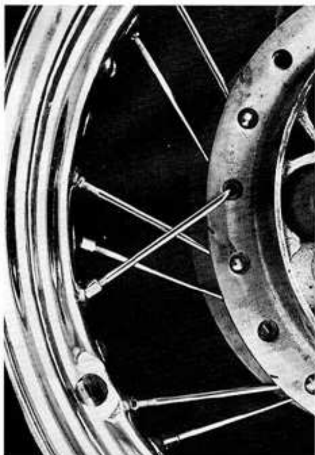
With this lacing method, outside spokes point off in counter direction.
