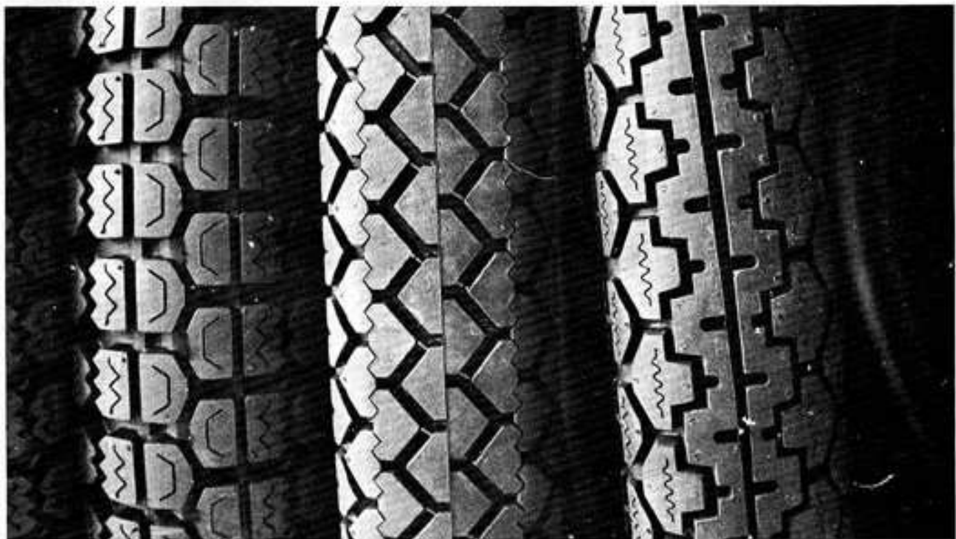
Left to right: Carlisle, Avon, and Dunlop. Both grooves and sipes show clearly in these tread patterns.
