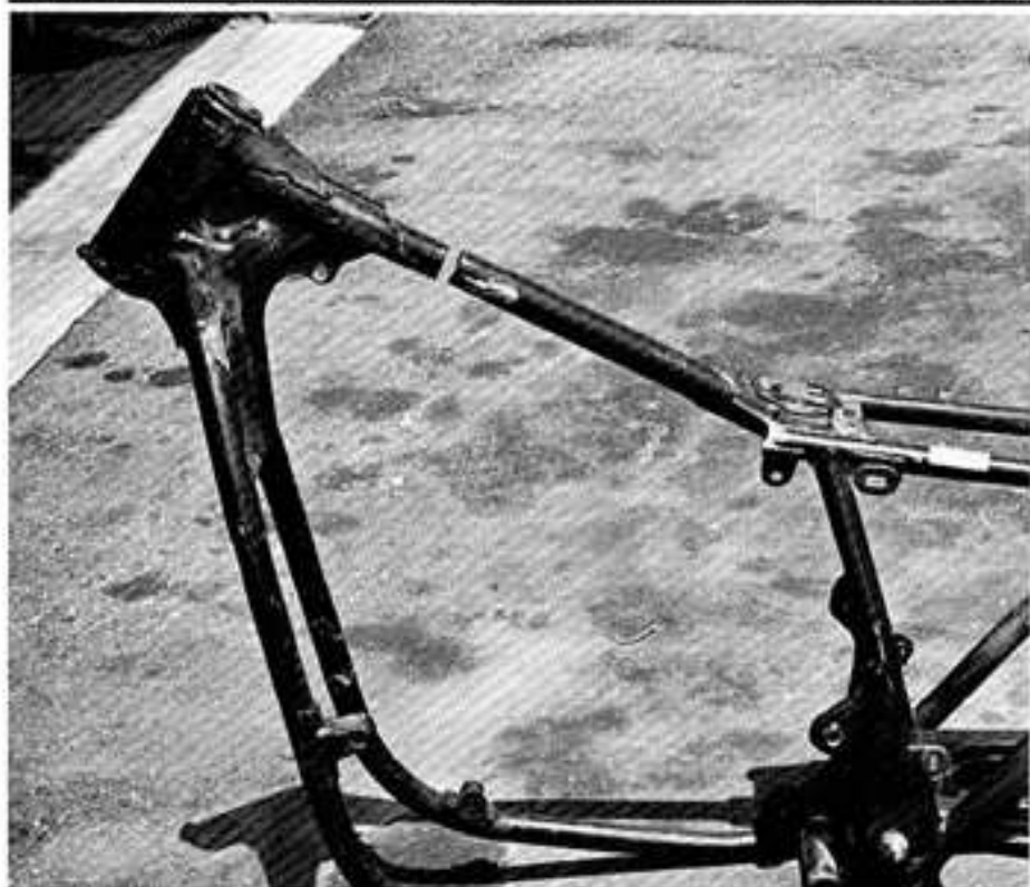
If more than \frac{1}{2} -inch is removed from top tube, it may be necessary to heat front down tubes and bend them.
