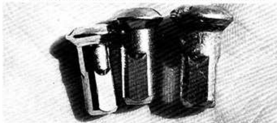
Nipples (10, 9 and 8 on right) will require different rim holes.
