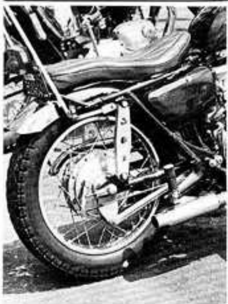
Struts made from flat aluminum stock are relatively easy to make and can be shaped as desired.
