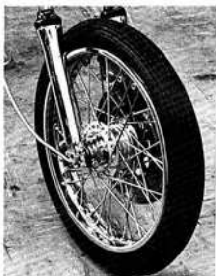
Drum brakes are best anchored to the rocker arm on springer front ends.
