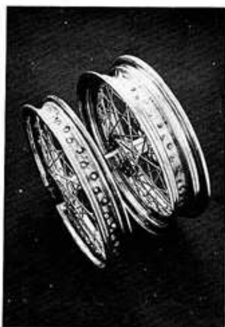
Difference between 4.00x18 and 5.00x16 (on right) is obvious.
