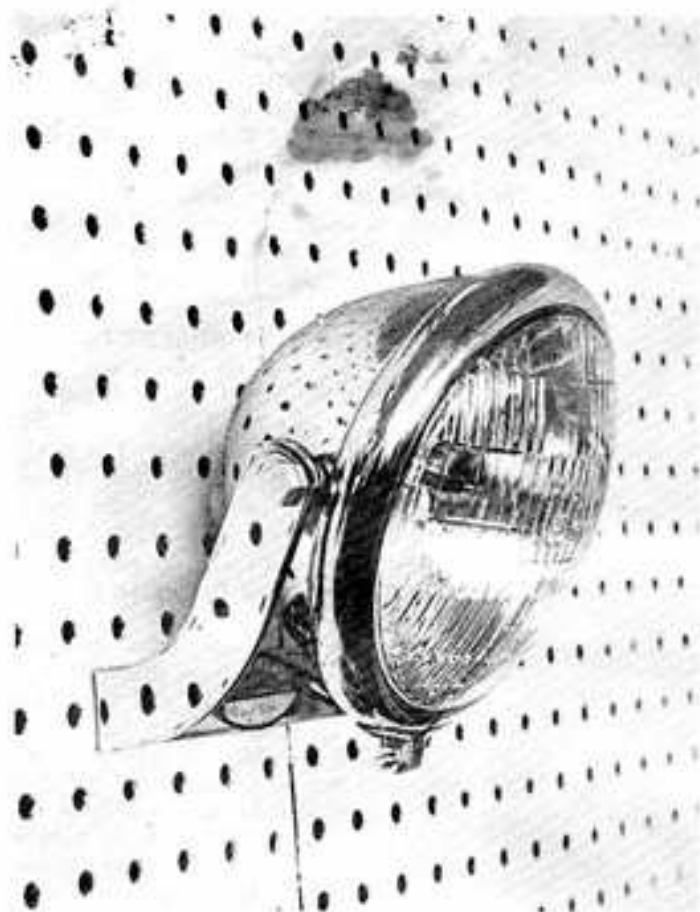
Ear type bracket works very well on extended standard forks and some springers and girders.
