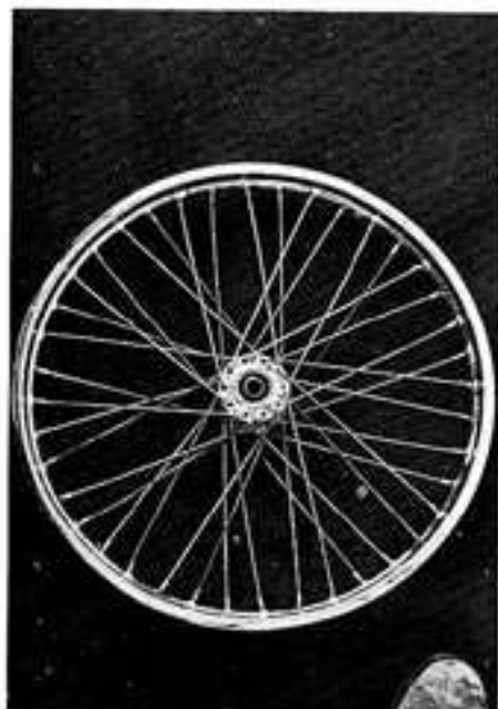
Spool hub and 21-inch rim laced together with cross-spoke style.
