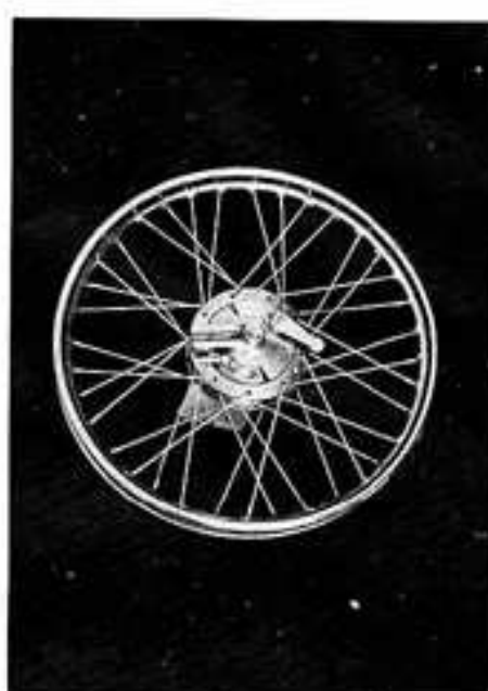
Any time a front brake is used, cross-spoke pattern is a must.
