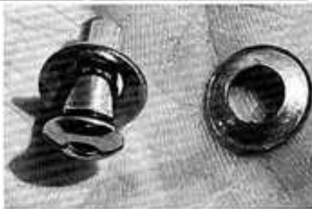
If rim holes are too big, a nipple washer can be used.
