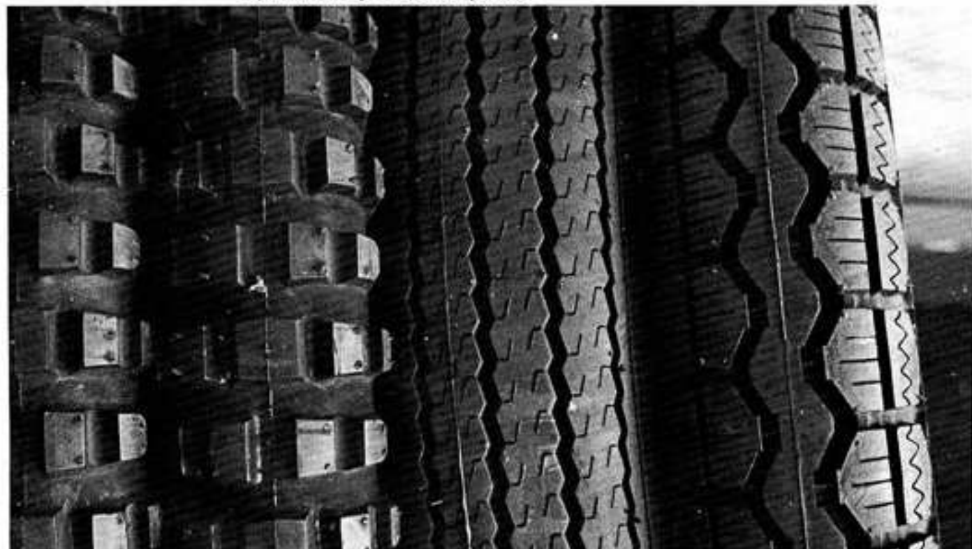
Knobby tread pattern on left may look mean but they aren't any good on pavement. Stick to normal patterns on right.
