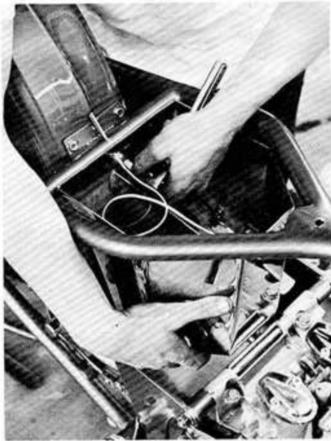
Honda 500 engine carries its own oil. Imitation oil tank holds electricals and tools.
