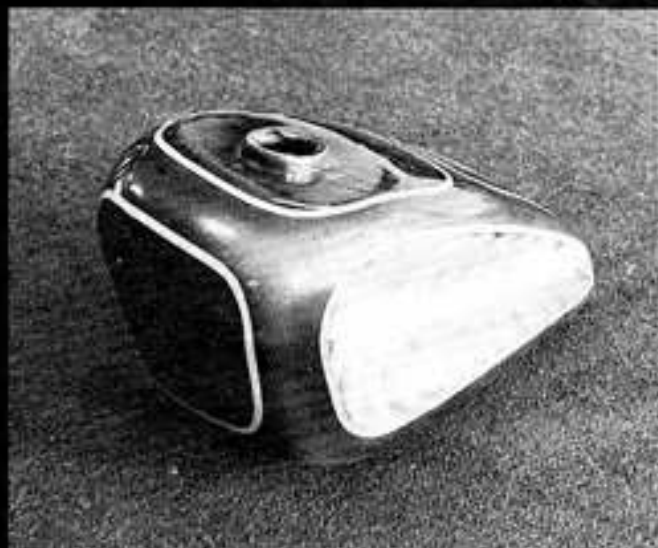
Popular Sportster style gas tank with concave sides and 'Frisco' type mount.
