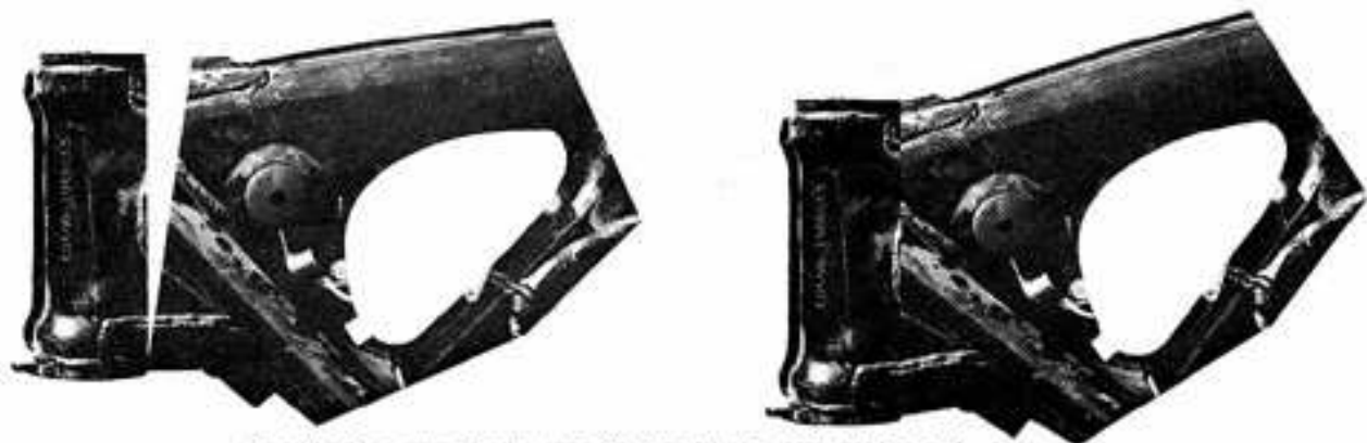
An alternative way to cut from the top of the neck section and remove a wedge. Weld the split up to finish it. It is easier to keep the steering head in line with this method.
