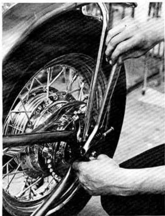
Always bolt fender, chain guard and sissy bar in before wheel is set in place. Easier that way.
